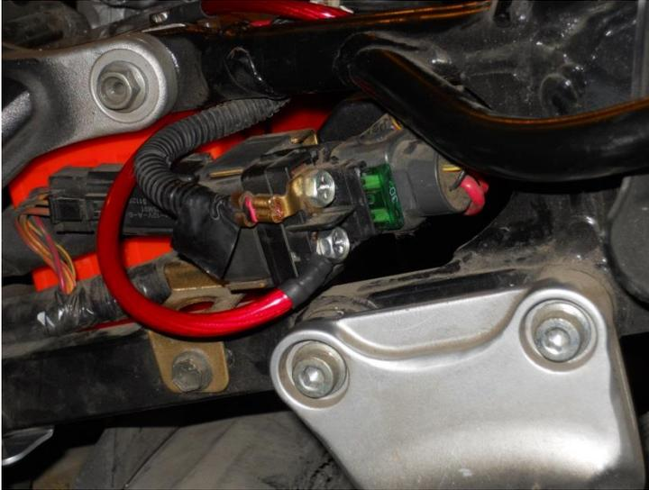
3. The longest 8 gauge wire will connect to the starter. Route the starter cable to the starter. Make sure it will not be pinched under the tank or along any other moving parts. Using the factory wire restraints under the tank, secure the new starter cable along the right side of the frame. Connect it using the factory nut/bolt on the starter, using the plastic boot left from the removed starter cable.
