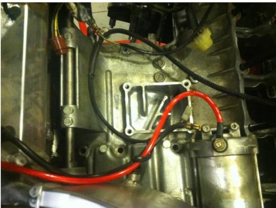
4. Remove the bolt from the negative (-) side of the primary battery and connect the single black wire to the negative side. Secure the bolt.
