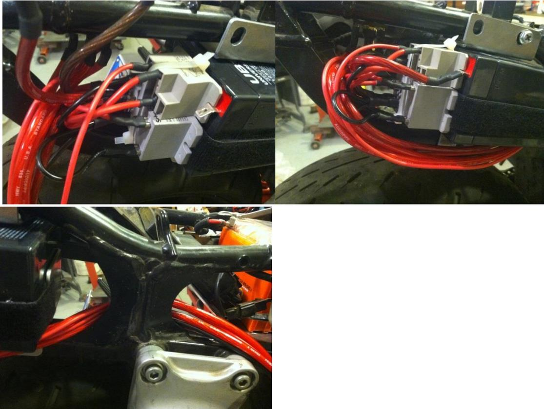
2. On the left side of the tail section, remove the plastic cover that protects the starter solenoid. Disconnect the starter cable from the starter solenoid (lower cable) and the starter. Remove the cable from the bike. Save the black plastic boot that covers the starter nut/bolt. It will be re-used when connecting the new starter cable. Route the shorter 8 gauge cable across the bike behind the battery to the starter solenoid. Connect it to the lower starter solenoid terminal as pictured.
