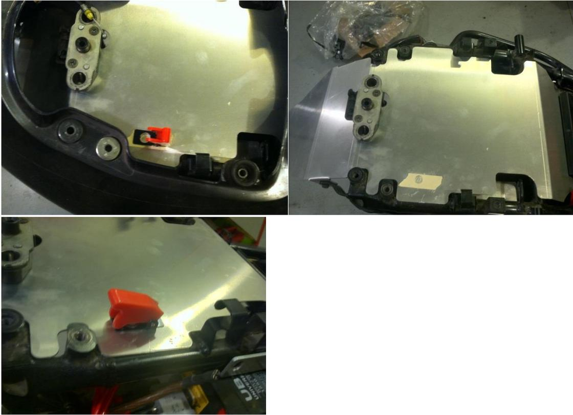
7. Lastly, connect is the longest thin wire. This wire must be connected to a switched ignition power source using the provided scotch-lock connector. This will allow charging of the secondary battery during operation of the bike. If connected to a constant 12v source, both batteries will slowly drain of power.
